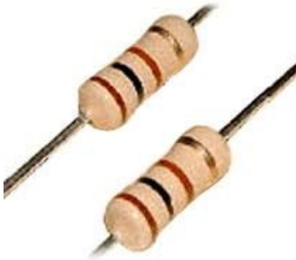
carbon resistor (see colour code p.115)
